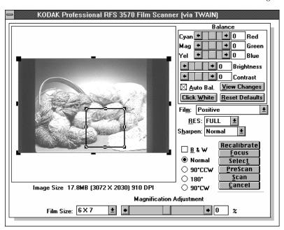
B. Click Focus. You will hear one buzz after another during the focusing process. A PreScan is done automatically once Focus is complete, and the image appears.
